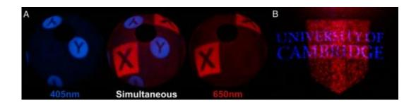
The new multicolored holograms offer a wide field of view, projecting images in 180°, which is better displayed on a sphere than on a plane. Credit: Montelongo, et al. ©2014 PNAS
