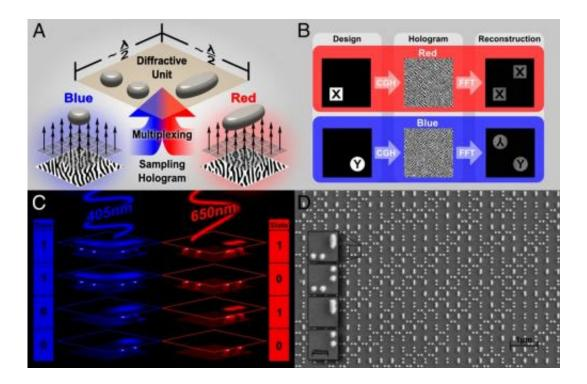
Different types of nanoparticles, which scatter light at different wavelengths, are used to create a multicolored hologram. Credit: Montelongo, et al. ©2014 PNAS
