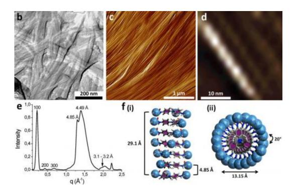
(b-d) Images of the organic metal, TATA, are shown with different imaging techniques. (e) X-ray scattering of a thin film of TATA. (f) Side view (i) and top view (ii) of the proposed stacking structure of TATA. Credit: Armao, et al. ©2014 American Chemical Society
