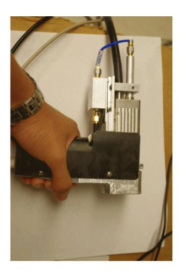
This is a photograph of the handheld probe. The motor, translation stage, ultrasonic transducer, and optical fibers are all incorporated in this handheld probe for easy operation. Credit: Yong Zhou
