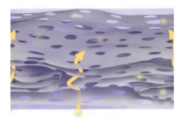
Close-up view of holey graphene framework film; arrows highlight ion-transport pathway short-cuts. Credit: UCLA
