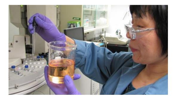
Non-toxic "green" propellant, actually peach-colored, is less harmful to the environment, increases fuel efficiency, and diminishes operational hazards. This class of propellant can replace highly toxic hydrazine and complex bi-propellant systems that are widely used today. Credit: Courtesy of Aerojet Rocketdyne
