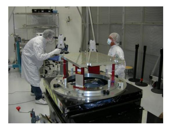
Ball Aerospace technicians use specialized equipment to build the GPIM satellite so that the space vehicle instruments and thrusters align perfectly with the payload interface. Credit: Courtesy of Ball Aerospace & Technologies Corp.
