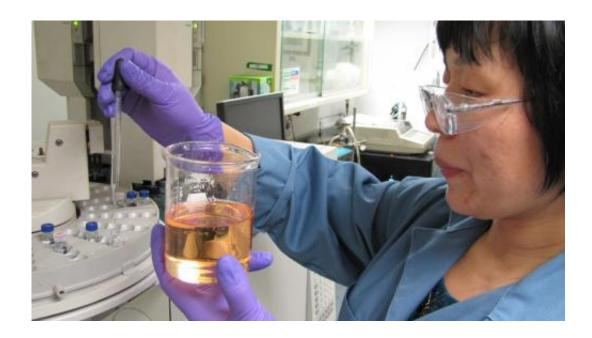
Non-toxic "green" propellant, actually peach-colored, is less harmful to the environment, increases fuel efficiency, and diminishes operational hazards. This class of propellant can replace highly toxic hydrazine and complex bi-propellant systems that are widely used today. Credit: Courtesy of Aerojet Rocketdyne
