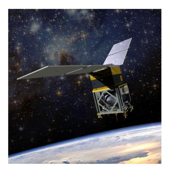
Artist rendition of NASA's Green Propellant Infusion Mission (GPIM) that will demonstrate and test the capabilities of a high-performance, non-toxic, "green" fuel on orbit. Credit: Image courtesy of Ball Aerospace & Technologies Corp.
