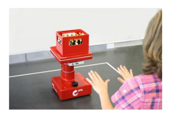
FiFi is controlled by gestures and carries small and big loads for the user. Credit: A. Trenkle / KIT
