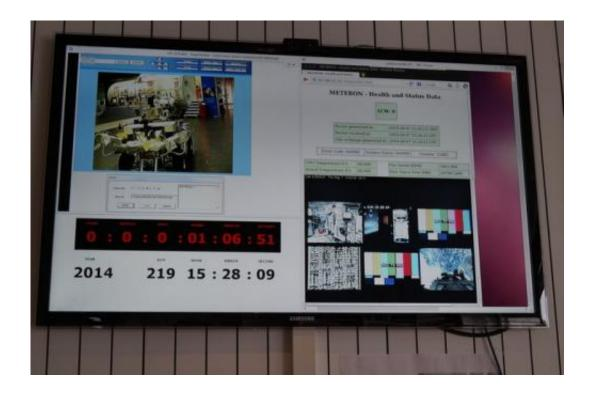
Screen showing live data flow between astronauts on the ISS and the Eurobot rover on Earth via the Meteron fault-tolerant next-gen network. Credit: ESA
