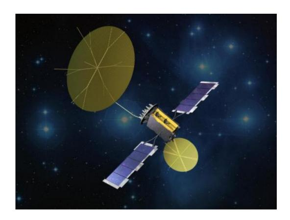
The fourth Mobile User Objective System (MUOS) satellite in the launch order is progressing in its final testing phase, having successfully cleared acoustic tests. This evaluation used powerful sound waves to simulate vibrations the satellite will experience during launch. Now the satellite moves on to thermal vacuum testing, which is the last step in its
