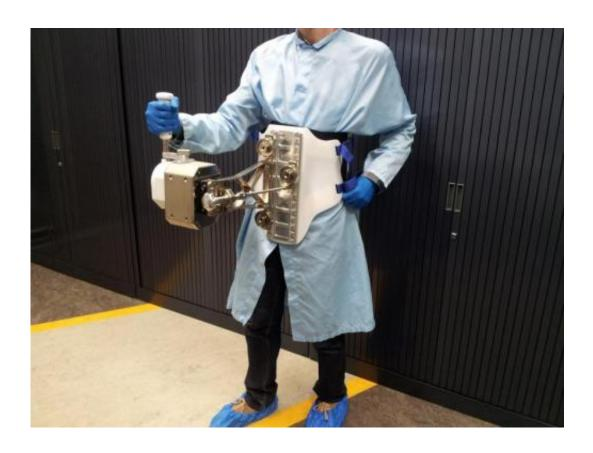
ESA's Haptics-1 body-mounted astronaut joystick will be used to investigate telerobotics for space aboard the International Space Station. Credit: European Space Agency
