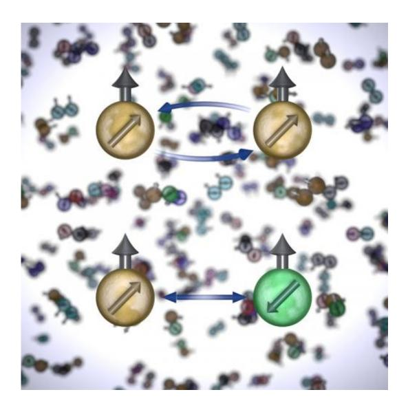
This is an illustration of symmetry in the magnetic properties -- or nuclear 'spins' -- of strontium atoms. JILA researchers observed that if two atoms have the same nuclear spin state (top), they interact weakly, and the interaction strength does not depend on which of the 10 possible nuclear spin states are involved. If
