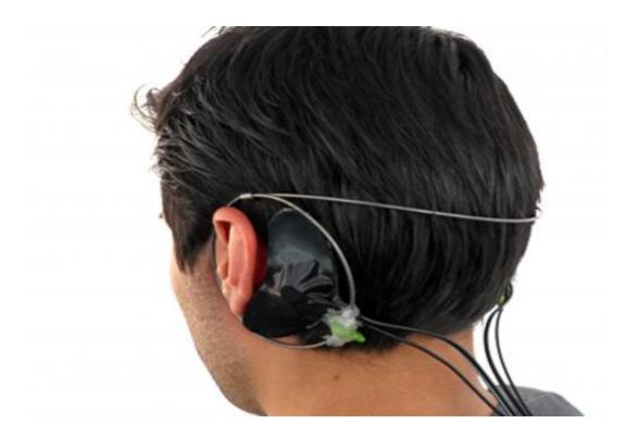
Specialists at the Monterrey Institute of Technology (ITESM) developed a device able to guide blind or visually impaired people in established routes through electrical stimulation of the organs associated with balance (vestibular apparatus).
