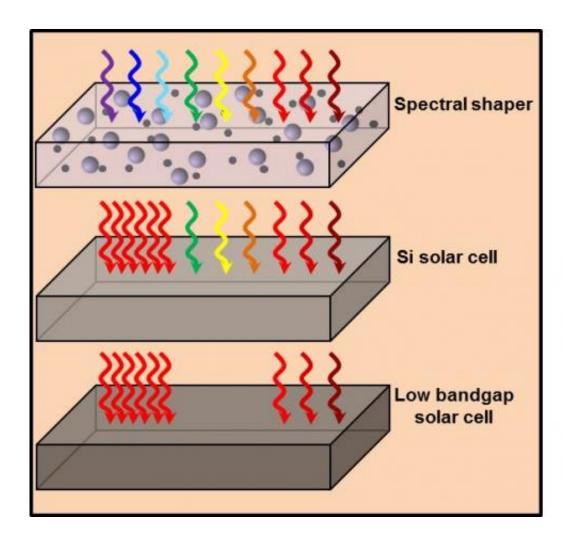
Potential use of a layer of silicon nanocrystals (large balls) and erbium ions (small balls) as a 'spectral shaper' for photovoltaic applications. This layer converts high-energy UV photons into infrared photons. These lower-energy photons are absorbed by an underlying solar cell. Credit: Fundamental Research on Matter (FOM)
