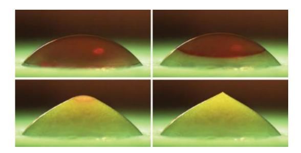
This image shows the freezing front, resulting in a pointy shape.
