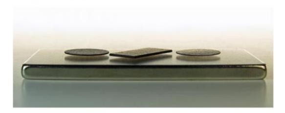
Three pieces of pyrolytic graphite are levitated freely over a single multipole NdFeB magnet
