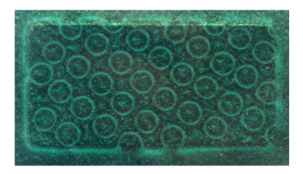
Magnetic field domain pattern of a printed multiple NdFeB magnet, revealed by magnetic field viewing film
