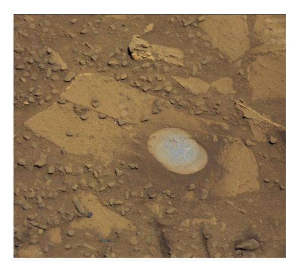
Curiosity rover used the Dust Removal Tool on its robotic arm to brush aside reddish, more-oxidized dust, revealing a gray patch of less-oxidized rock material at a target called "Bonanza King," visible in this image from the rover's Mast Camera (Mastcam). Credit: NASA/JPL-Caltech/MSSS
