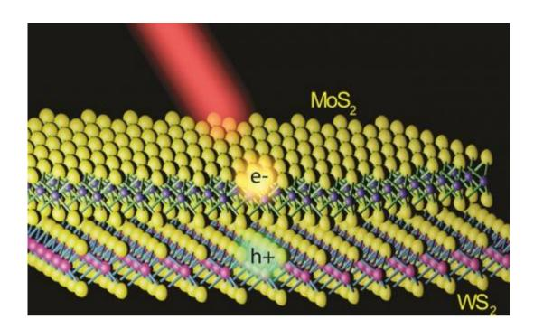
This is an illustration of a MoS2/WS2 heterostructure with a MoS2 monolayer lying on top of a WS2 monolayer. Electrons and holes created by light are shown to separate into different layers. Credit: Feng Wang group, Berkeley Lab/UC Berkeley
