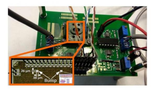
Experimental setup and chip micrograph.
