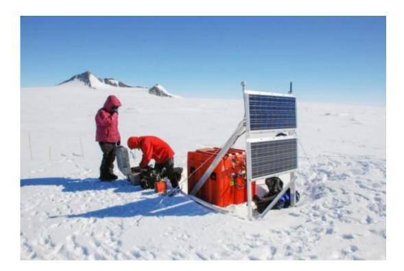
The HOWD Polenet seismic station is located near the northwest corner of the Antarctica's Ellsworth Mountains. It was the station that showed the clearest indication of high-frequency signals following the 2010 Chilean earthquake. Credit: Eric Kendrick/Ohio State University
