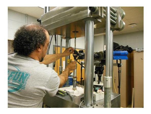
John Chumack of the University of Dayton Research Institute's structural integrity division prepares a material sample for high-rate tensile testing.
