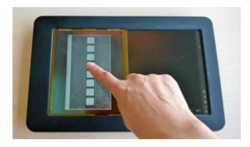
An electrostatic haptics prototype on which the gray area feels rough, like sandpaper, and the dotted line has a notched texture for scrolling.
