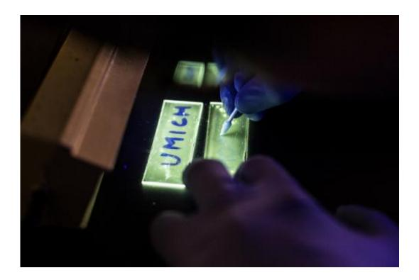
The phosphorescent LEDs can reveal the presence of water under backlight. Water causes polymers to break in the LEDs, changing from phosphorescent light (green) to fluorescent light (blue). Credit: Joseph Xu
