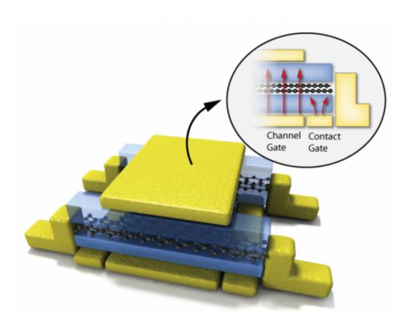
An illustration of the novel geometry that enabled measurement of the tunable fractional quantum Hall effect in bilayer graphene. Credit: Columbia University
