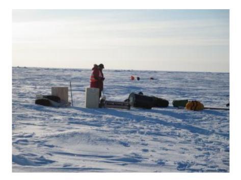
A scientist assembles an ice-tethered water profiler on the ice in March. The instrument is now anchored in a hole in the sea ice, with a moving piece to measure the water properties below. Credit: M. Ohmart, Univ. of Washington
