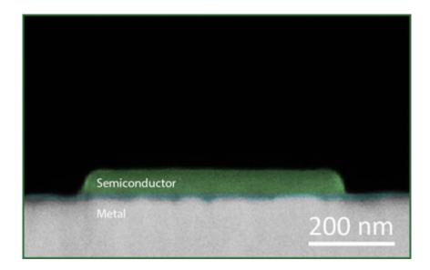
The scanning electron microscope shows the semiconductor (made of cadmium sulfide) on top of the metal surface (silver). Credit: Ren-Min Ma and Sadao Ota
