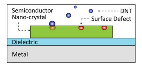
The plasmon laser sensor consists of a 50-nanometer-thick semiconductor separated from the metal surface by an 8-nanometer-thick dielectric gap layer. Surface defects on the semiconductor interact with molecules of the explosive DNT. Credit: Ren-Min Ma and Sadao Ota
