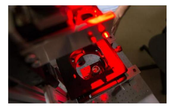
"Unlike most techniques, which study lots of molecules at once, with these magnetic tweezers we are looking at one DNA molecule at a time," explains Andresen. "These so-called 'single-molecule' techniques are at the cutting edge of biophysics research, allowing us to understand how a single DNA molecule might behave in our bodies."
