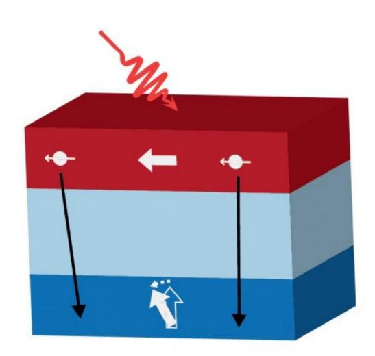
A simplified representation of the new technology is shown. Two magnetic layers, each with a different magnetization, are separated by a neutral layer. A laser pulse strikes electrons in the upper layer. This causes them to move through the material, in the direction of the second layer. The spin of these electrons, in the direction of the magnetization of the upper layer, exerts a force on the spin of the electrons in the lower layer to make them rotate in the same direction.
