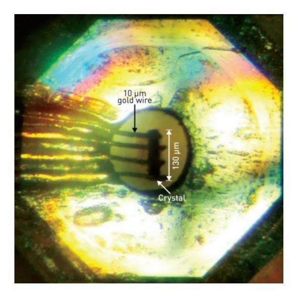
The diamond anvil cell used to induce superconductivity in a single-component nickel–organic molecule. Credit: Reproduced, with permission, from Ref. 1 © 2014 American Chemical Society
