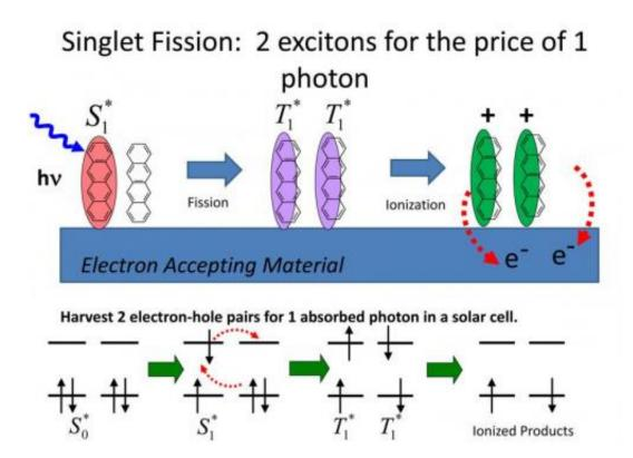
Singlet fission is a process in which a single photon generates a pair of excited states. This 1->2 conversion process has the potential to boost solar cell efficiency by as much as 30 percent. Credit: Bardeen Lab, UC Riverside.
