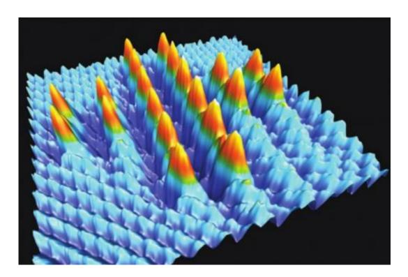
20 bromine atoms positioned on a sodium chloride surface using the tip of an atomic force microscope at room temperature, creating a Swiss cross with the size of 5.6nm. The structure is stable at room temperature and was achieved by exchanging chlorine with bromine atoms. Credit: Department of Physics, University of Basel
