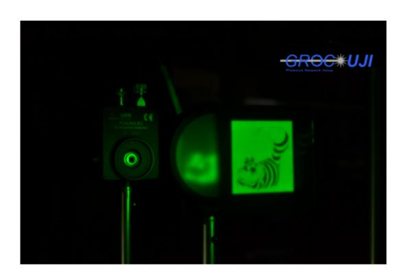
The researchers placed an image of the Cheshire Cat in front of a scattering layer that completely hid it, then used the image they were able to retrieve from photodetected values recorded by the photodiode to demonstrate that disorderassisted imaging can indeed recover an object's fine details -- even using a sensor without spatial resolution. Credit: Jesús Lancis/Jaume I University.
