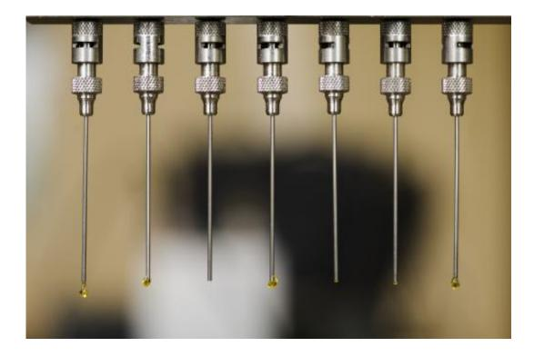
Fibers begin forming near the ends of tiny nozzles in a UA laboratory set-up. The researchers are refining a new material to potentially extract uranium from the ocean for use in nuclear power. Credit: Jeff Hanson
