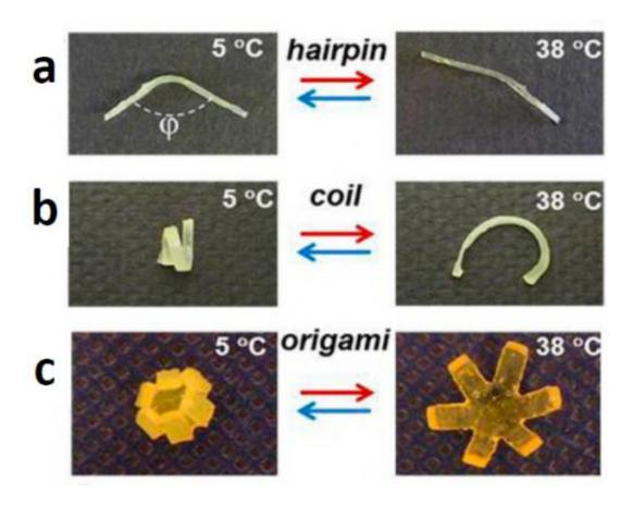
Examples of two-way reversible shape memory (a-c) demonstrated by polymers.
