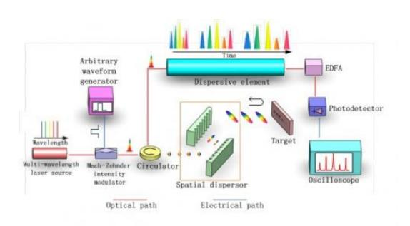
This is the experimental setup of the STEAM system for ultrafast imaging based on a multi-wavelength laser. Credit: Science China Press
