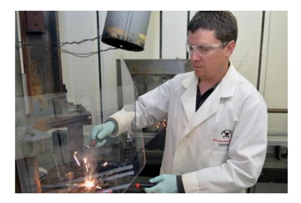
Los Alamos National Laboratory chemist Bryce Tappan ignites a small quantity of aluminum nanoparticle water mixture. In open air, the compound burns like a Fourth of July sparkler.
