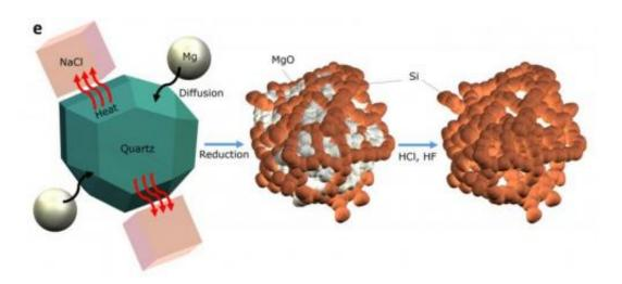
A schematic showing how sand is turned into pure nano-silicon. Credit: UC
