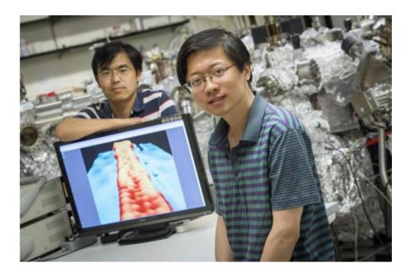
Yaoyi Li (foreground) and Mingxing Chen, UWM physics postdoctoral researchers, display an image of a ribbon of graphene 1 nanometer wide. In the image, achieved with a scanning-tunneling microscope, atoms are visible as "bumps." Credit: Troye Fox, UWM Photo Services
