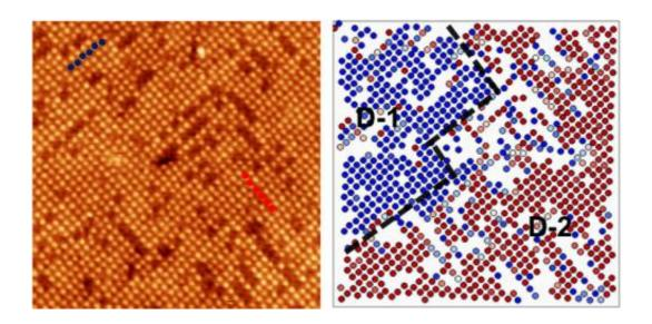
An Oak Ridge National Laboratory study combined microscopy and data processing to provide an unprecedented look at the surface of a magnanite material known for its unusual properties. The resulting "distortion maps" (right) brought into view structural areas called domains that were not easily identified in the raw images (left). Credit: ORNL
