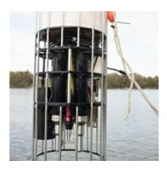
A unique water profiling instrument developed by The University of Western Australia's Centre for Water Research (CWR) is enabling scientists to understand the impact of even the most subtle turbulence on algal populations.
