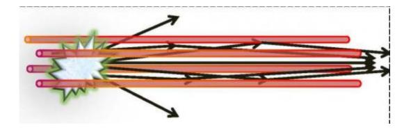
This is an illustration of an air waveguide. The filaments leave 'holes' in the air (red rods) that reflect light. Light (arrows) passing between these holes stays focused and intense. Credit: Howard Milchberg
