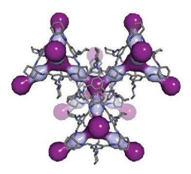
In this computer simulation, light and dark purple highlight the cavities within the 3D pore structure of CC3. Credit: *Nature Materials* 2014
