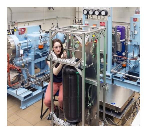
NIST's Jodie Pope and her team have developed this prototype field test standard to test the accuracy of hydrogen fuel dispensers. Credit: Suplee/NIST
