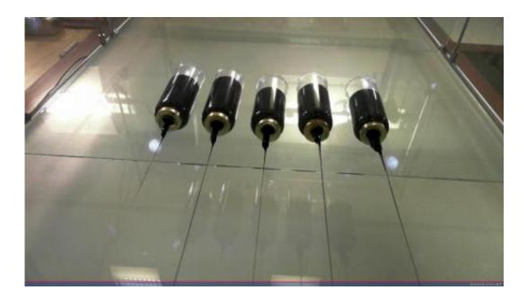
Queen Mary University of London have set up five bitumen samples in glass tubes with different orifice diameters. Two webcams record the samples by taking the pictures from top and bottom angles every hour. An image is taken at 10am everyday -- this is a photo from the bottom camera taken on Wednesday 25 June. Credit: Queen Mary University of London
