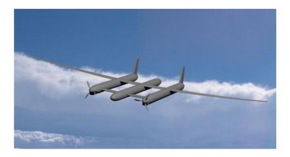
Taking second place, the team at Purdue University in West Lafayette, Indiana, designed the OQ451-5 Trident, a hydrogen-powered UAS capable of seven days of uninterrupted flight. Credit: Purdue University
