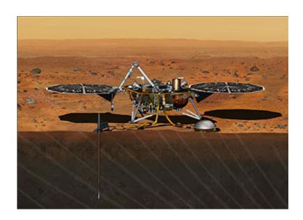
Artist's impression of the InSight Mars lander. The SEIS will be deployed onto the surface using a robot arm, where it will then record signals from marsquakes and meteorite impacts in order to probe the planet's interior. Credit: NASA/JPL-Caltech
