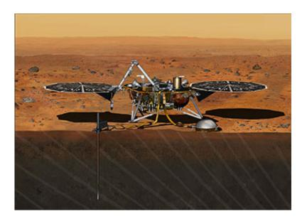
Artist's impression of the InSight Mars lander. The SEIS will be deployed onto the surface using a robot arm, where it will then record signals from marsquakes and meteorite impacts in order to probe the planet's interior. Credit: NASA/JPL-Caltech
