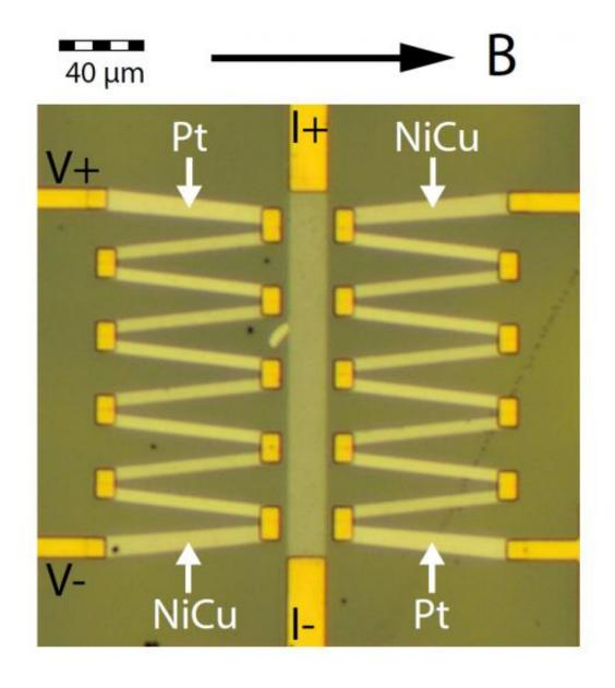
The sample used for the measurement. In the middle, from top to bottom, is the platinum strip. Electrons move through this strip and produce a spin current in
