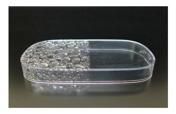
A nanoparticle-based coating from ARS, applied to the right half of this plastic container, prevents water from beading and reducing visibility. Credit: Sanghoon Kim.
