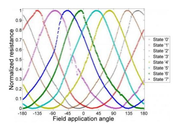
This graph depicts measured signal during a reading operation for all eight possible states of a 110-nm, 3-bits, self-referenced MRAM cell. Credit: Quentin Stainer
