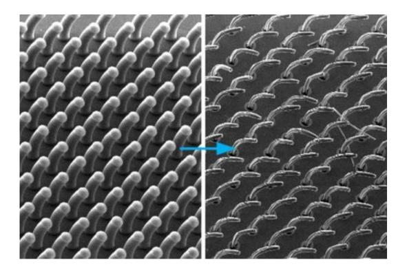
New process developed by MIT's John Hart and others can produce arrays of 3-D shapes, based on carbon nanotubes growing from a surface. In this example, all the nanotubes are aligned to curve in the same direction.
