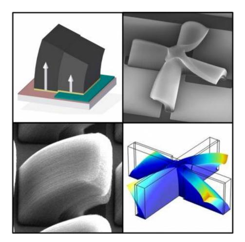
Close-up microscope images of carbon nanotube forms and illustrations of the patterns that produce them. At left, a simple curved form, and at right, complex curved propeller shapes, that can be produced by this carbon nanotube growth method.
