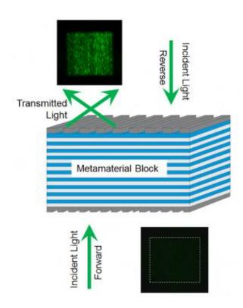
This is a schematic of NIST's one-way metamaterial. Forward traveling green light (left) or red light passes through the multilayered block and comes out at an angle due to diffraction off of grates on the surface of the material. Light traveling in the opposite direction (right) is almost completely filtered by the metamaterial and can't pass through. Credit: Xu/NIST
