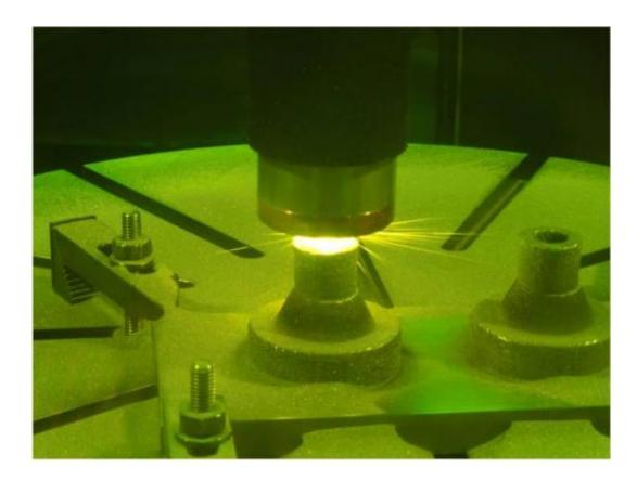
Scientists make a rocket nozzle using a new 3-D printing technique that allows for multiple metallic properties in the same object. Credit: NASA-JPL/Caltech
