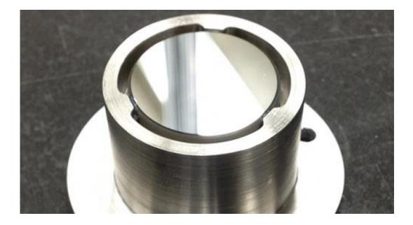
This is a prototype of a mirror mount that scientists made using a new 3-D printing technique. Credit: NASA-JPL/Caltech
